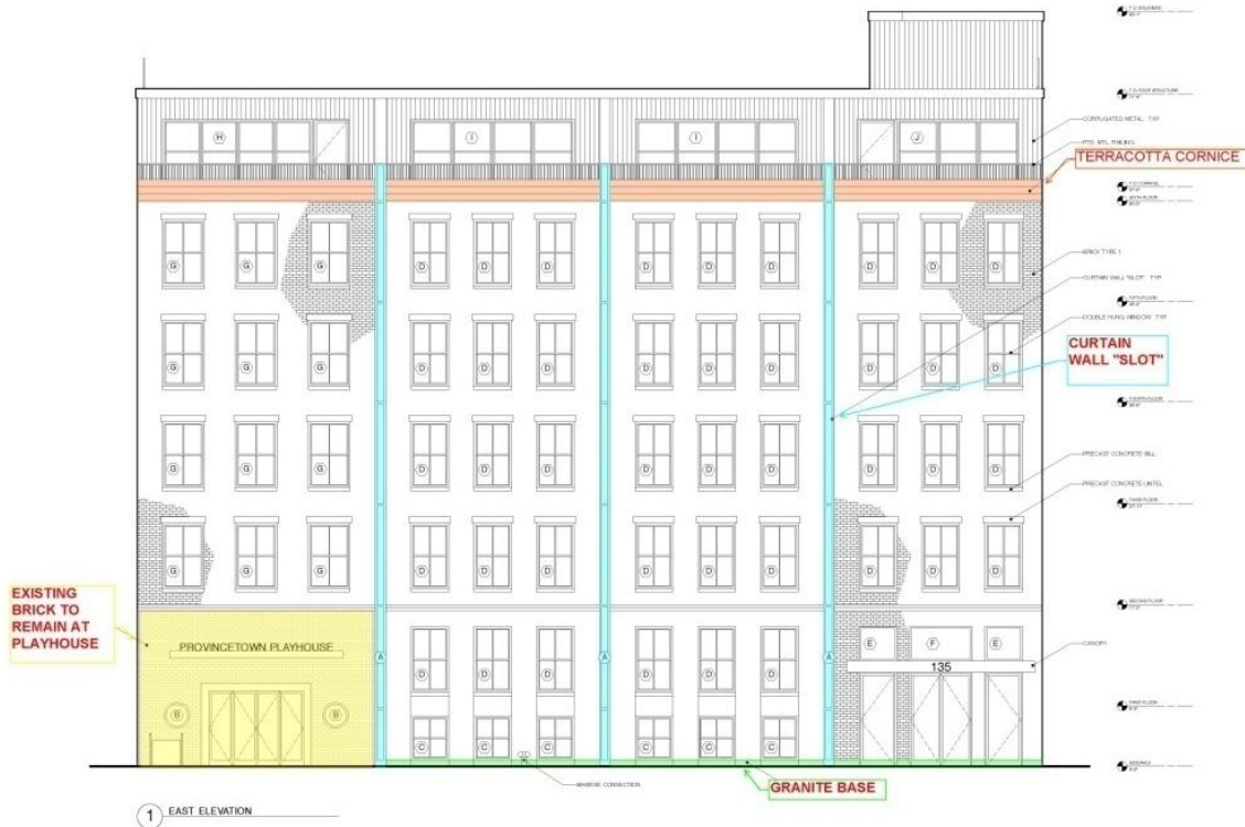
Figure 12: Shows the Three Curtain Walls Slots, Granite Base, Existing Wall to remain, and the Terracotta Cornice
